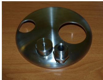
Tack weld 304 S/steel assy ready from brazing
