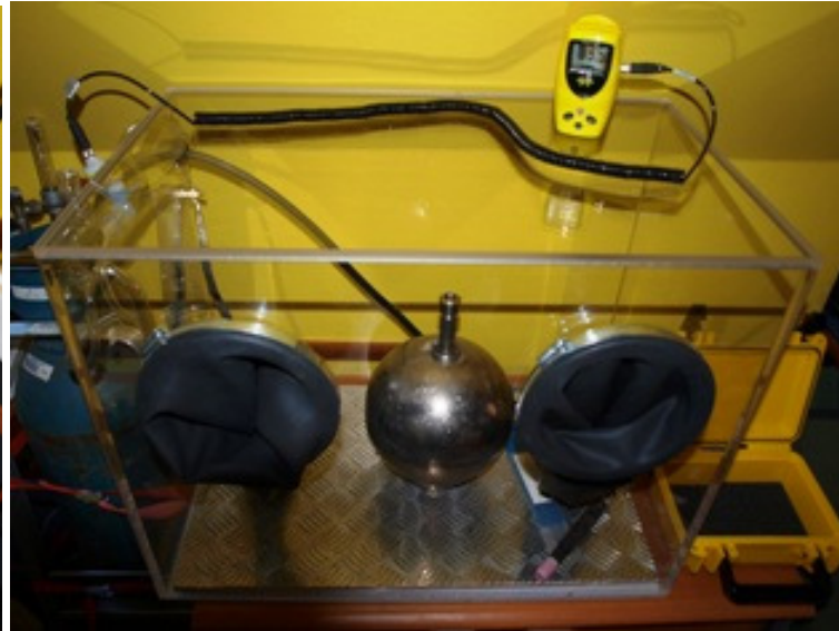
Argon atmosphere welding glovebox with O 2 sensor picture shows titanium sphere ready for welding
