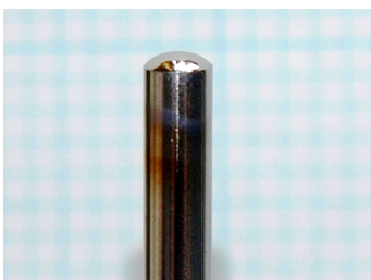
4mm tungsten pin with nickel dome
